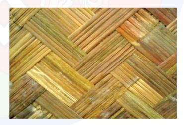
Bamboos are flattened by hammer, (or now- a-days, in some parts of the country, they are left on the road for vehicles to run over them). These flattened straps of bamboo are woven into different patterns; usually alternating the inside-out and outside in. These mats are used for making sheds and huts. These types of mats serve as pre-fabricated materials for constructing outdoor VIP camps and large public meeting halls.
